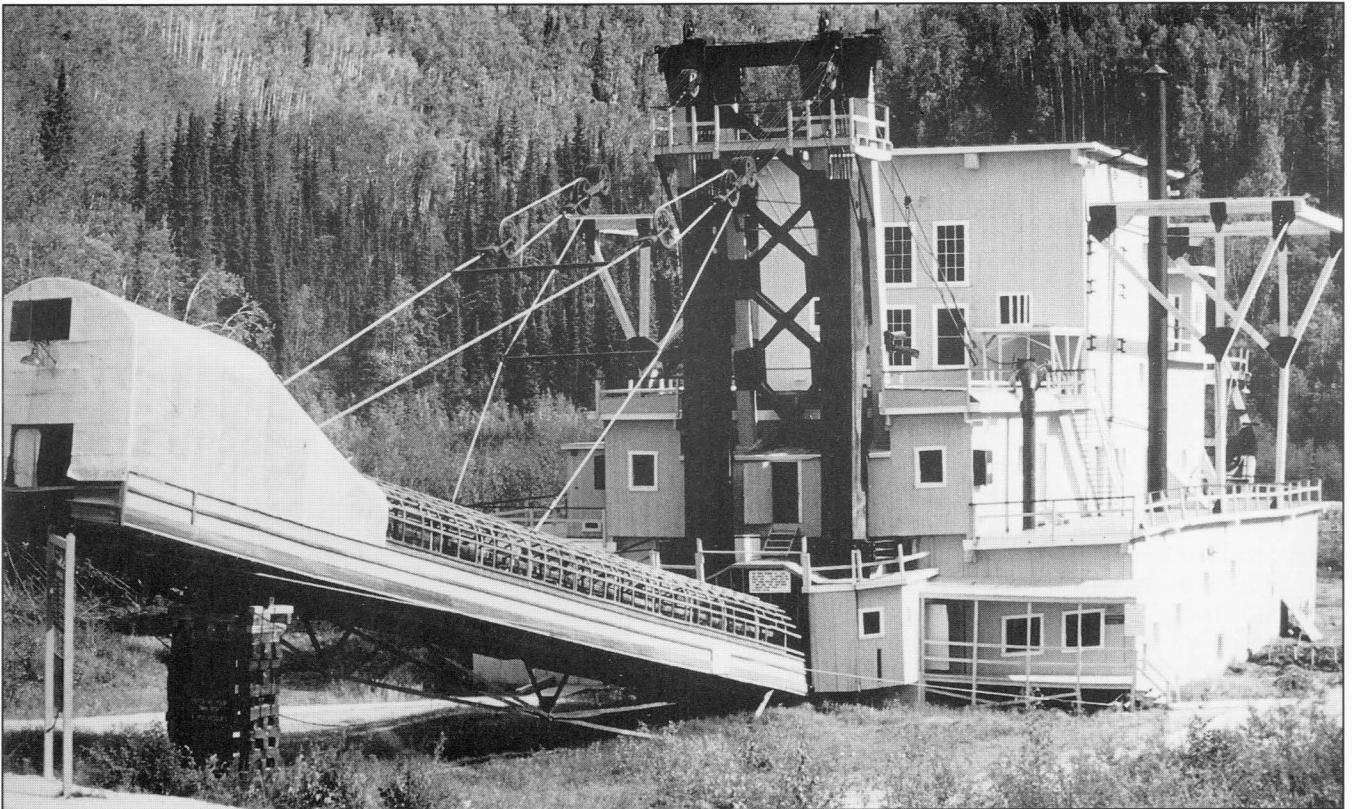
Fig. 10. Dredge Number 4, preserved on Bonanza Creek where it ceased mining in 1959. The long arm houses the tailings conveyor belt, and the bucket chain is out of sight at the far end. The photograph was taken in 1990, before the dredge was completely dug out of the gravel and turned around (photo by the author).
